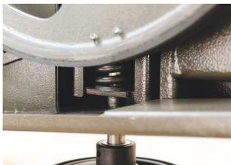
▲ The heavy tension spring is just visible behind the cast band wheel
